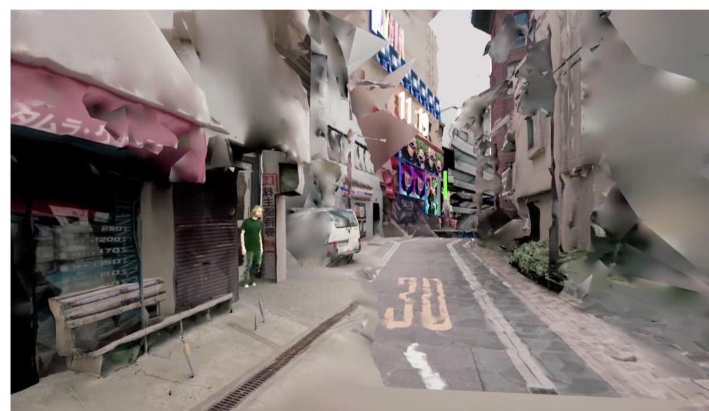
Fig 10. 'Current' reconstruction without deep learning to fill in data voids on city texture mapping.
